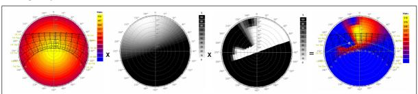
Figure 5 A diffuse radiation factor can be determined by multiplying the diffuse sky distribution by both incidence angle and shading factors for each sky segment.
