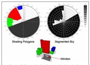
Figure 2 Example shading masks for window centre, showing shading polygons (left) and the sky dome divided into discrete segments (right).
