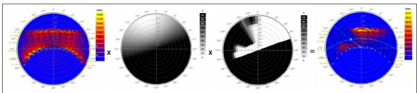
Figure 6 Total solar collection can be calculated using a cumulative sky, in which solar radiation through each segment is aggregated over time and then multiplied by incidence angle and shading factors.
