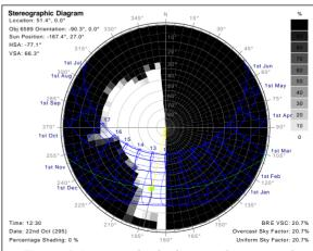
Figure 1 An example shading mask generated for an overshadowed window in London mapped over a sun-path diagram.
