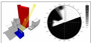
Figure 3 Shading masks for planar surfaces must store fractional shading information.
