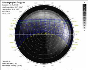
Figure 10 An example shading mask for an internal floor surface with windows along the northern and eastern facades.
