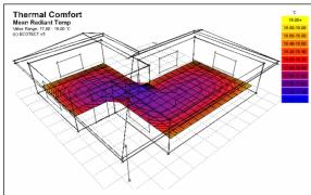
Figure 11 Shading masks can be modified to include object proximity data for dynamic radiant temperature and comfort calculations.
