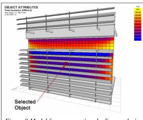
Figure 8 Model for comparative shading analysis.
