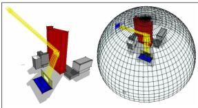
Figure 9 It is also possible to calculate and store reflected solar radiation in a shading mask.
